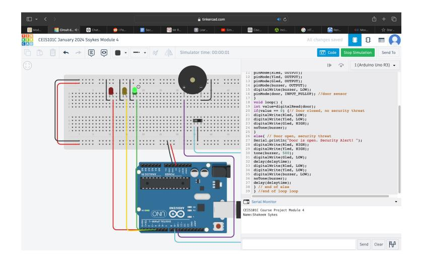
Circuit of door open with Green LED OFF (picture)
